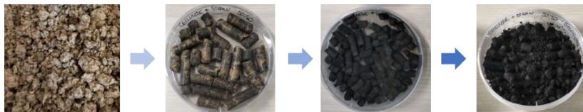
Fig. 1. From left to right: raw cellulose, mixed pellets, carbonized pellets and biologically activated biochar.
